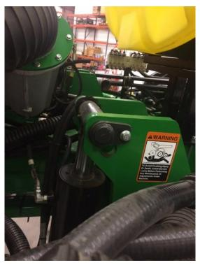
When lifting the planter for the first time after installing or changing any pins using the "translift" function use caution and watch the area in the red oval as the barrel of the lift cylinder may contact here. If this happens double check which holes you used for your cylinder pins on the top and bottom of the lift cylinders.
