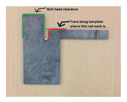
The photo below is showing the area marked out to be cut and ground off.
