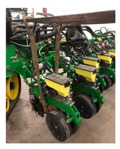
4. Once unit is in place, install bottom mounting bracket and leave a little slack to allow side to side movement of unit for proper placement. Be sure to measure row width to achieve proper row unit placement before tighten bolts.
