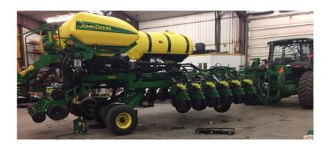
2. With planter weight supported on jack stands begin removal of the existing axle assembly.
