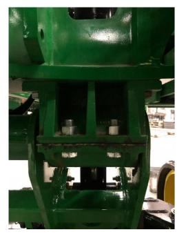
6. Insert flag pin through cylinder lift eyes and fasten retaining bolt on flag. On older DB planters the factory pin is too short, if your pin is not 10 inches of effective length a new one should have been included with your kit. MAKE SURE YOUR PIN IS LONG ENOUGH TO GO THROUGH ALL THE PLATES ON THE LIFT ARM!!! On a DB44 planter we use a plain pin and trunnion blocks bolted into the lift arm on the track axle instead of a flag pin.
