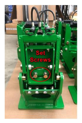
9. Once the bracket bolts, set screws and jam nuts are tightened down, row unit and row tip installation is completed.
