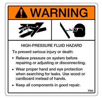
Hydraulic fluid that is escaping under pressure can have sufficient force to cause injury. Confirm all hoses and connections are always in good working order by looking over daily. Failure to do so may result in serious personal injury or death. Escaping hydraulic fluid under pressure may have enough pressure to perpetrate skin causing serious injury. Avoid this hazard by relieving the pressure before disconnecting lines or servicing the system.
