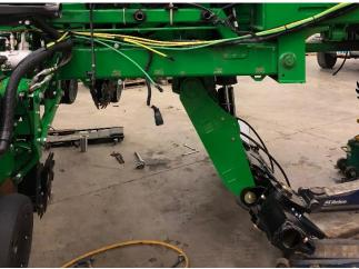
4. Align side to side to be sure lift cylinders line up with mounting tabs on axle assembly.
