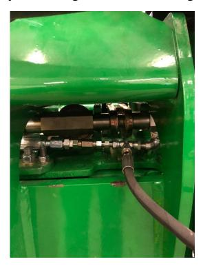
7. When installing the small cylinder ensure to install it on the side that has the most clearance.
