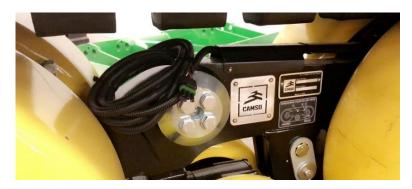
If you do not have a harness coming from your front idlers you will need to remove speed sensor from the wheeled axle assembly. Sensor will be installed in new tone wheel assembly on the right front idler wheel of the track undercarriage.
