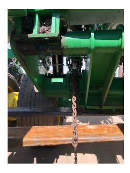
8. Axle assembly can now be removed from underneath the planter. A forklift with forks spaced to carry the outside tire works well for sliding the assembly out from underneath the planter.
