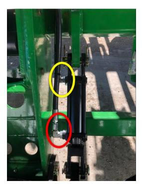
Picture to the left is the left side main lift cylinder, pictured to the right is the small rock cylinder located on the lift arm.
