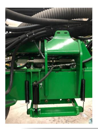
8. After mounting the row tip on the planter wing, and adjusting the proper spacing to the row beside it, lock the set screws and jam nuts located on the underside of the assembly to keep the unit from sliding side to side. Jam nuts are shown in the bottom view.
