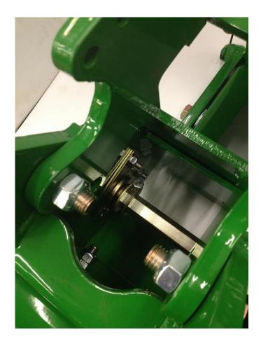
In order to retract the drive dog close enough to the row on narrow row planters, it may be necessary to mount the hex bearing on the inside as shown in the photo above to the right. If that is the case put the clamp on the inside as shown in the picture to the right.
