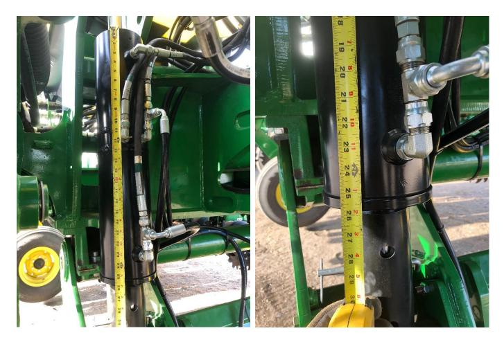
**Note:** Floor jack can aid in re-alignment of the pin hole of cylinder rod to axle ears.
