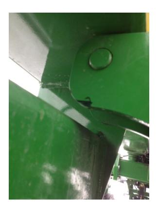
1. First begin by removing the top plate of the row tip. Remove the bolts, sprigs, and small cylinder in order to slide the row tip into place on the planter.
