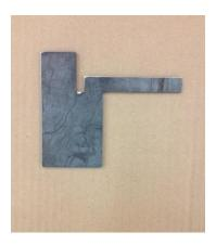
We have found some of the newer DB planter frames have less clearance in the bracket that mounts a roller. Use the gauge to see if your planter has enough clearance for the row tip to fit. With the planter folded up hold the template up to your roller brackets resting the long narrow part on top of the 7x7 tube and holding the template tight to the front side of the tube, see photos below.
