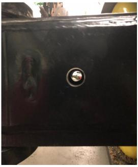
3. Slide bolt into hole and tighten provided lock nut to secure tracks to axle assembly.
